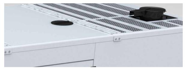
All roof joints are reinforced with lap joints utilising butyl rubber seals, providing excellent protection against water ingress in extreme conditions. Curved edges ensure a rigid and aesthetically pleasing enclosure structure. The radiator is accessed via a flush mounted rain cap with compression seal – a further guard against water ingress.
